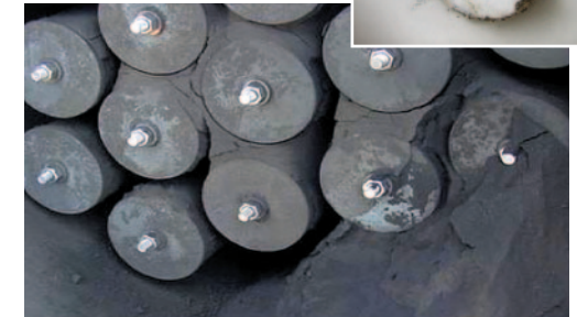
Old standard elements — inefficient and prone to surface blinding (top photo)
